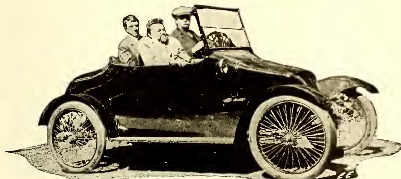
The New Gasoline-Electric Automobile Which Its Inventor—Harry E. Dey, Seen at the Wheel,—Expects to Sell at $500.00. At the Left—Dr. Charles P. Steinmetz, the Famous Electrical Engineer, Who Believes Mr. Dey has the Best Idea Yet in Electric Automobiles. The Storage Battery is Charged While Running.
