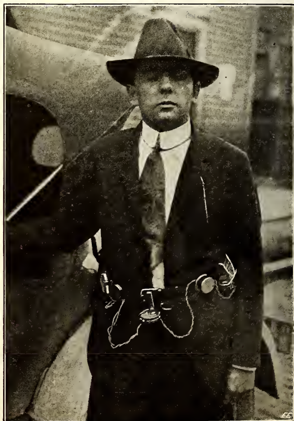
The Electric Direction Indicator, Worn by its Blind Inventor, Who Developed It to Enable Him to Get About Without a Cane. The Specially Constructed Compass is Worn in Front. The Two Metal Projections, One on Each Side of the Compass, Are the Buzzers. Clasps at the Sides of the Belt Hold Two Triple Cell Batteries, Which Supply the Current for the Device.
